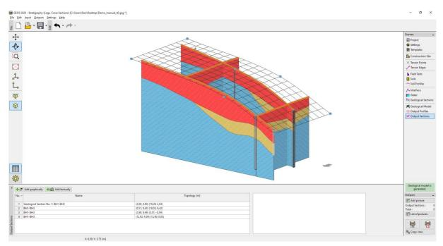
Created sections can be copied into other GEO5 programs. We will open the created section and copy the section to the clipboard by clicking the "Copy output section to Clipboard" button.
