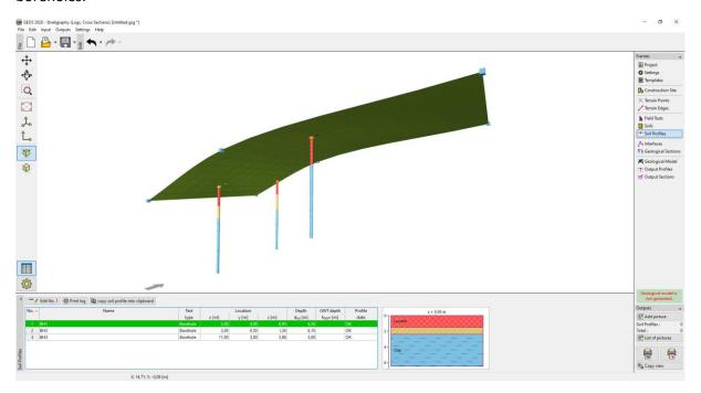
Note: The reason for the existence of Soil profiles is similar to that of "Soils". Complex and detailed boreholes need to be simplified for the geotechnical model. Penetration tests (CPT, SPT) can be interpreted into geological profiles too. This can be done either in this frame or when making geological sections. Creation of earth profiles from field tests is described in EM number 43 – Creation of Soil profiles from Field tests.
