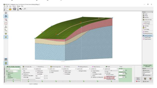
The created model of the subsoil can be further modified using new boreholes. For example, we assume that the landfill layer on the front side will be constant. We can make this adjustment by adding a new borehole.
