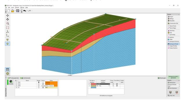
In the "Output sections" frame, we can enter any number of sections in the model. This view can be very clear and useful.
