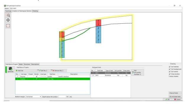
By clicking the "Generate" button, we can verify the input by generating the soil areas.
