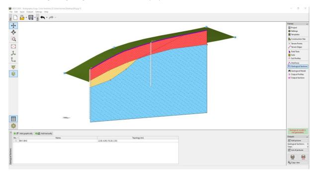
In the "Geological Model" frame we select the "Master Borehole". Mater borehole determines the number and the order of soils in the model. This borehole has to contain all of the soils in the model. In the table, we assign the interfaces, that we had defined during the creation of the Geological section.
