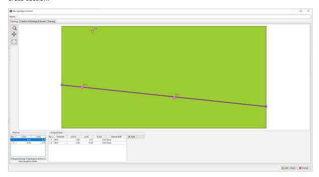
Note: Geological sections are a basic element when creating a 3D subsoil model. Here you can draw your idea of layers. The 3D model will then respect your assignment. Tests and ground profiles that do not pass through the section can be displayed as well.
