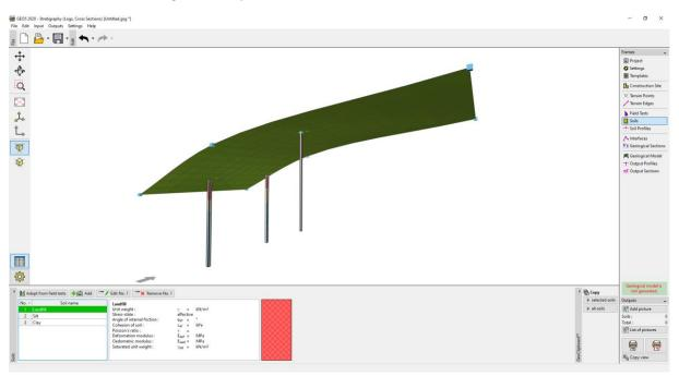
Note: In a real geological survey we can have a large number of soils with minimal differences. For a geotechnical model, it is suitable to merge these soils into a "Geotechnical type" and work with those. The soils (geotechnical types) that we input here will be used not only in a 3D subsoil model but will be transferred to other GEO5 programs too.
