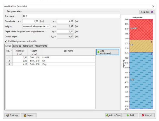
When inputting the second and third borehole, we can either copy the first borehole and edit the layer thickness or re-enter the borehole and only assign the already entered soils from the catalog.
