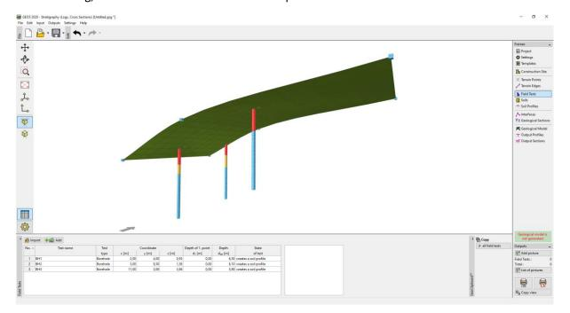
In the "Soils" frame, using the "Adopt from the field tests" button, create a soil list.
