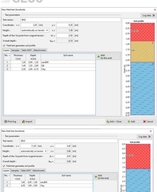
Note: For a real borehole, we usually enter a much larger number of layers and descriptions. We can also enter the information about the water, taken samples, upload photos and other attachments. Description of how to create borehole documentation is in the EM no. 42 – Creation of Field Test Documentation.
