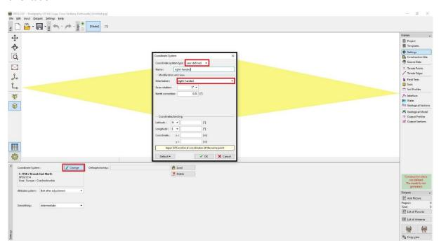
Note: For real constructions, the coordinate system used in the given country or region is selected. In the Czech Republic, it is the JTSK and all coordinates are then added into this coordinate system.
