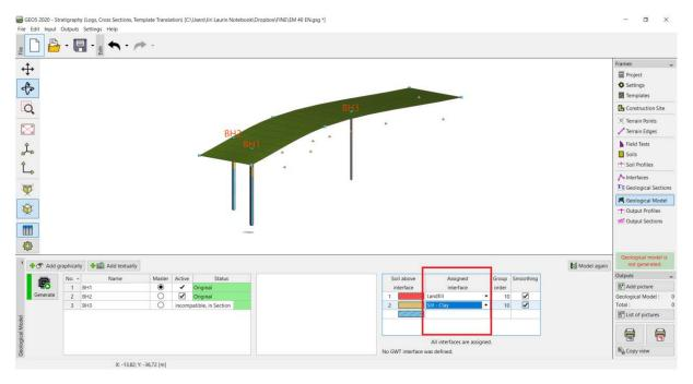
Note: Master borehole must contain all soils (or soil layers), that are present in the model - even those that are not physically in the area of this borehole. This is common when we create a model with lens or faults. For more information, view EM 41– Advanced Modeling in the Stratigraphy Program.
