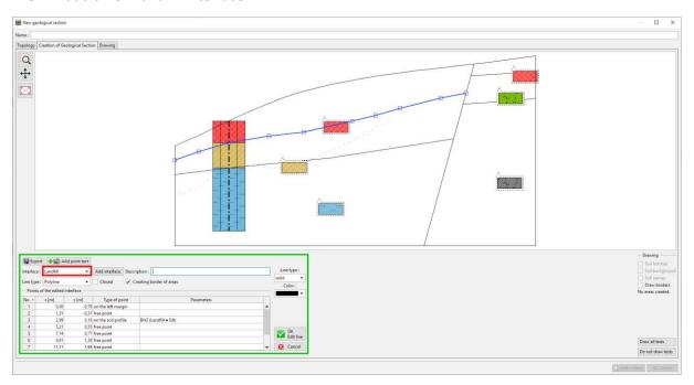
Note; The 3D model is only affected by points that have assigned interfaces. If we want to keep the exact shape of the interface in the 3D model, we might need to model the interface by more points – even if the section is straight.
