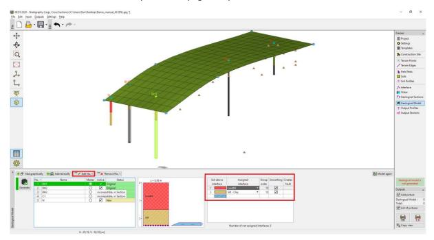
We will open the window for editing the master borehole and add new soil behind the fault (from top to bottom). As we do not know the position of the layer interface in the borehole (or there is no interface at all), we will leave the location type as "not defined"
