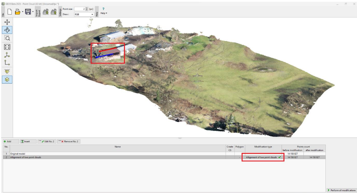
Aligned point cloud
