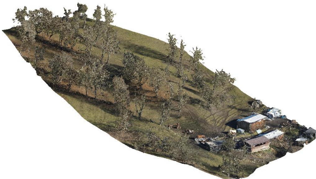
Point cloud 1 – upper part of the slope focused by photogrammetry
